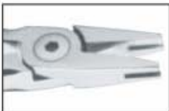
DE-1400 "V" bend stop special design makes 1mm "v" bends to shorten archwires or provide a positive stop. Excellent for placing stops in titanium wires. For round or rectangular wires up to .025"
